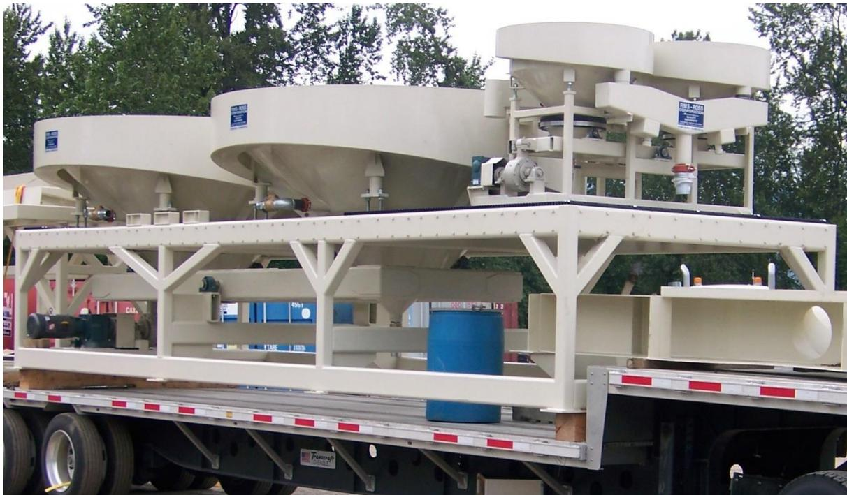
Circular jigs are more efficient than trapezoidal or square configurations where interference patterns result in zones of pulse disruption, negatively affecting feed flow. Whereas pulsations occurring in a concentric round chamber, working at a tuned frequency, will give rise to balanced nodal pulse patterns providing even vertical sorting of the jig bed. Therefore, the RMS Circular Jigs are more efficient by inherent physical design.
