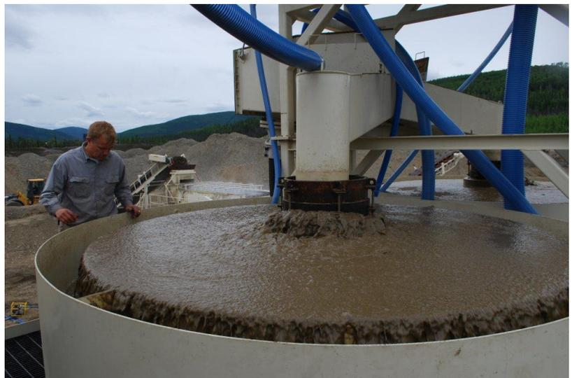
In conventional square jigs, the feed accelerates toward the discharge. However, in circular jigs the feed decelerates as it approaches the discharge because the cross sectional area of the flow channel increases dramatically as the feed approaches the discharge. Therefore the particulate retention time is substantially longer in the RMS-Ross CIRCULAR JIG compared to any traditional jig, enhancing the capture of fine gold.
