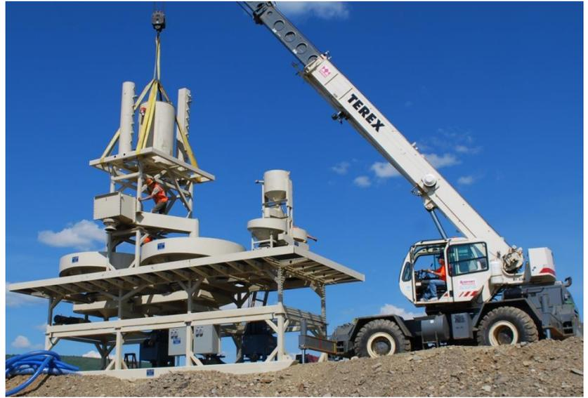
JIGS, also known as mineral jigs, are one of the most widely applied gravity concentrating devices used in the world. They are widely used as concentrators for recovery of tin, heavy rare earths, diamonds, gold and platinum group metals.
